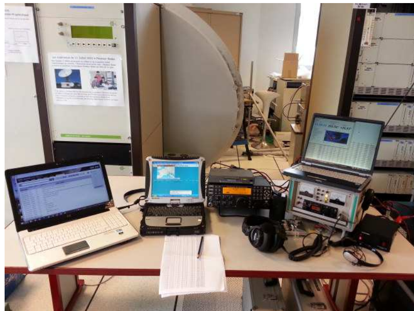
K3 + 432/28MHz tvr + doppler shift compensation
