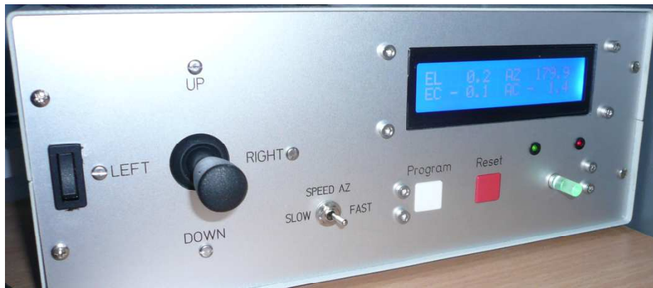
Station de pilotage El. et Az.
