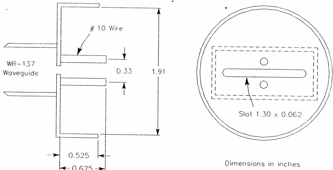
Fig 2—Clavin feed for 5760 MHz.
