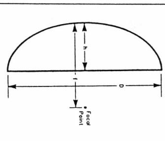
Fig. 9—Measure the proportions of your dish and calculate the location of the focus as described in the text.
