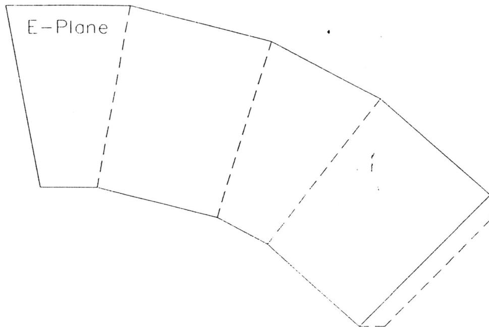
Fig 3—Full-size template for a 7.2-dBi horn for 5760 MHz, suitable for illuminating a dish with  $f/D \approx 0.47$ .
