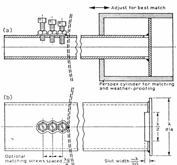
Fig 161. A simple feed for dishes having an f/D ratio of 0.25–3. Matching can be done either by matching screws as shown or as in (a) by using a Perspex matching (and weatherproofing) sleeve. (b) Side view of feed
