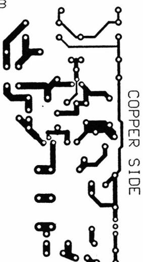
Frequency Doubler from 2.5 GHz to 5 GHz using GaAs FET
